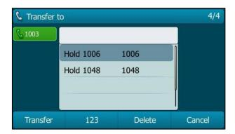
3. Press  $(o_K)$ ,  $(o_{TRAN})$  or the **Transfer** soft key to complete the transfer.
