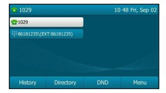
The following figure shows an example of label display when the label length feature is set to Default:
