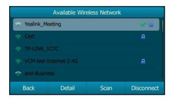
**3.** Press the **Detail** soft key to view the detailed wireless network information (e.g., Profile Name, SSID or Signal Strength).
