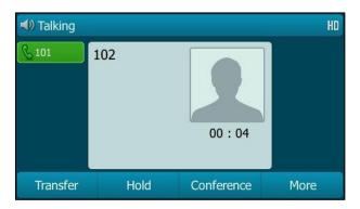
If the park retrieve code is configured, press the **Retrieve** soft key on the dialing screen or retrieve key (if configured) on the IP phone.
