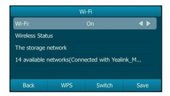
When Wi-Fi USB dongle WF40 is connected to the USB port at the back of the IP phone, the LCD screen will prompt "Wi-Fi adapter has been added, scanning the available wireless network right now?". You can Press the **OK** soft key to activate Wi-Fi mode directly and scan Wi-Fi devices automatically.
