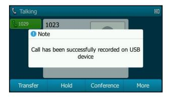
Press the **Start REC** soft key to start recording again, the recording will be saved in a new ".wav" file.
