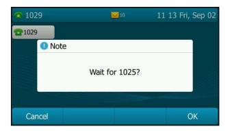
**1.** Press the **OK** soft key, the phone returns to the idle screen and call completion is activated. When the called party becomes idle, the following prompt will appear on the LCD screen of the phone:
