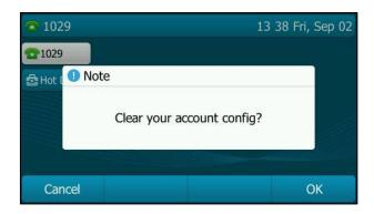
**2.** Press the **OK** soft key, registration configurations of all accounts on the phone will be cleared immediately.
